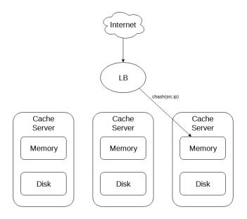
L4 load balancing, backend selection based on IP
